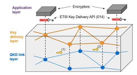
AES Encryptors are an off-the-shelf technology, already widely used in telecom (using non quantum safe key exchange)
